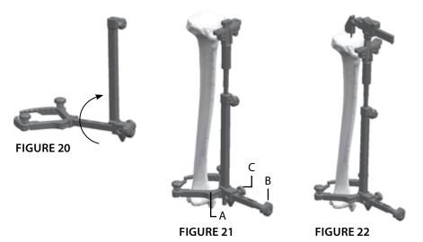
into the center of the proximal tibia, adjust the internal-external rotation of the guide, then drive both spikes into the tibia with a mallet. | FIGURE 22
